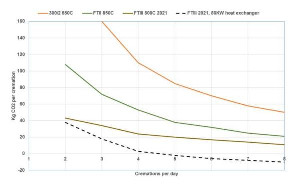
The performance figures indicate that not only is the new FTIII more energy efficient in its use of gas than the current equipment operated but also significantly reduces the level of gas consumption the more cremations per machine are undertaken. The method of operating one cremator and maximising number of cremations per day was adopted in 2023 as reported to the Joint Committee, this approach reduced gas usage and resulted in significant savings.
